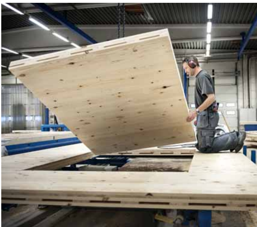
A CLT panel consists of three to eleven layers, always an odd number, of laminations glued together.
