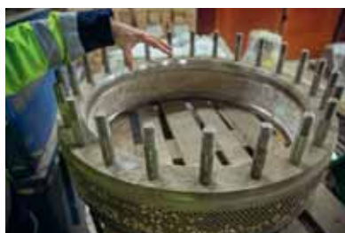
Pellets are manufactured by sawdust being pressed through about 3,000 holes in the press matrix.
