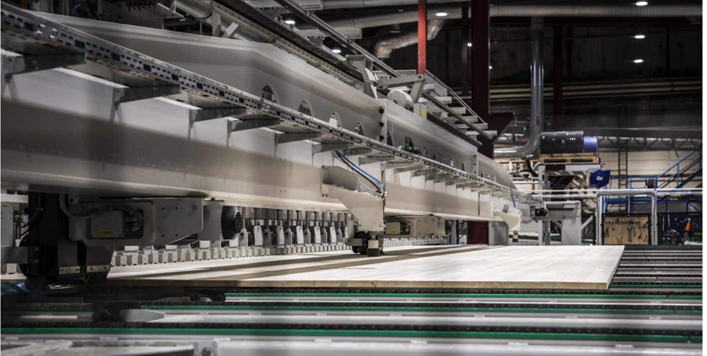
With its enormous 6 x 20 metre press table, the glue press in Långshyttan is one of the largest in the world.
