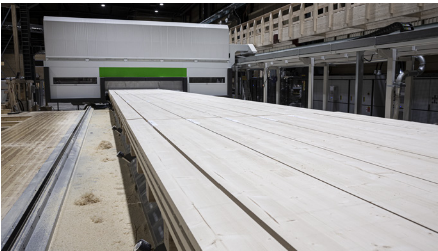
The computer numerical control (CNC) machine handles everything from precision work to rougher cuts in the crosslam sheets.
