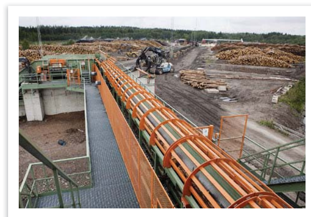
Hasselfors is a high-production and flexible sawmill that earns praise for both quality and delivery reliability. The picture shows the intake to the reducer bandsaw.
