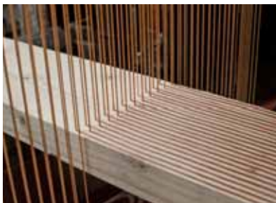
Wood laminates pass through a curtain of glue with high strength and durability.
