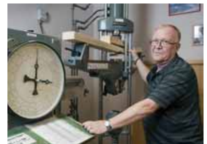
The strength of finger joints and the quality of the laminate joints are tested regularly.
