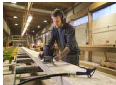
At inspection, the beams are checked and visible damage is repaired.
