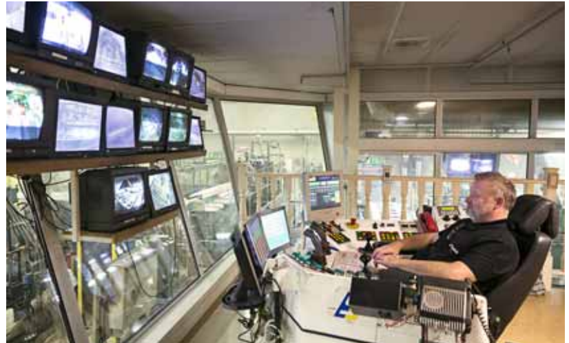
Mats Boman sits in the control room and monitors the entire sawing process. Via screens he controls the flows so that production moves in an optimal manner.
