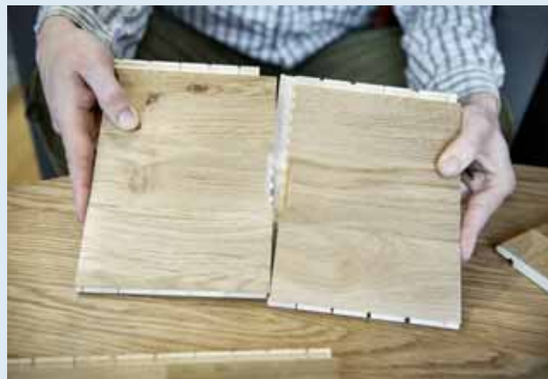
The multilayer parquet board was invented in 1941. Today’s modern parquet has a special locking function which counteracts movement in the wood.
