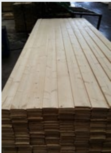
The length of the finished product is set to 3.985m which gives a few centimetres to play with when the 12-metre long container is loaded.
