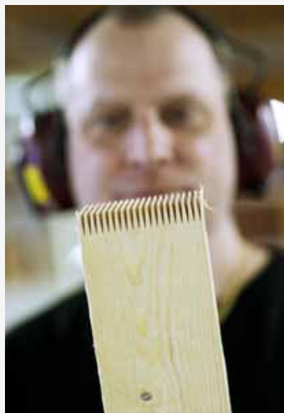
The milled fingers are critical to getting a tight and stable joint.
